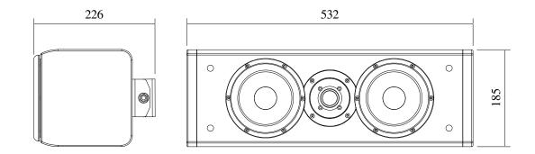
**SYSTEM**: 2 way vented box loudspeaker.
